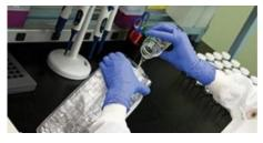
Step 3 Seal in Quanti-Tray Sealer and place in  $35^{\circ}\text{C} \pm 0.5^{\circ}\text{C}$  incubator for 24 hours.
