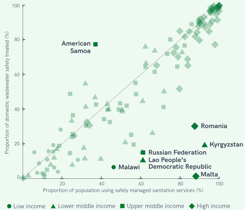
FIGURE 66 Comparison of SDG indicators 6.2.1a (safely managed sanitation services) and 6.3.1 (safely treated wastewater, domestic fraction) for 2022
